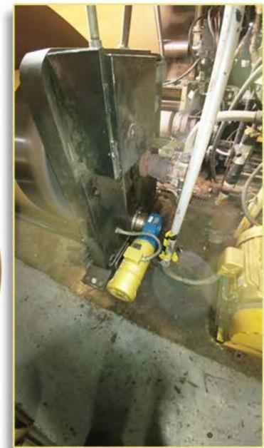
■ Motor and reduced ratio gearbox for smooth wrap arm performance.
