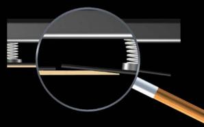
When running certain widths of board, some systems allow the outer feet to tilt causing edge crush and delamination.
